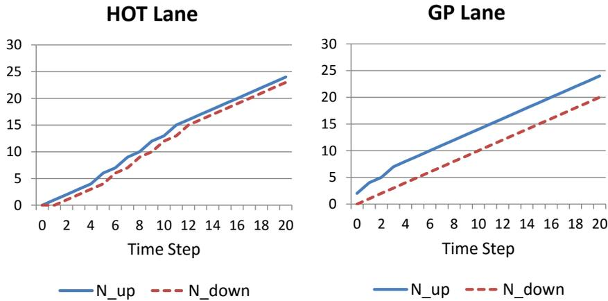
Figure 5.5:  $N$  value plot for the HOT and the GP lanes for simulation 2 revenue maximization objective
