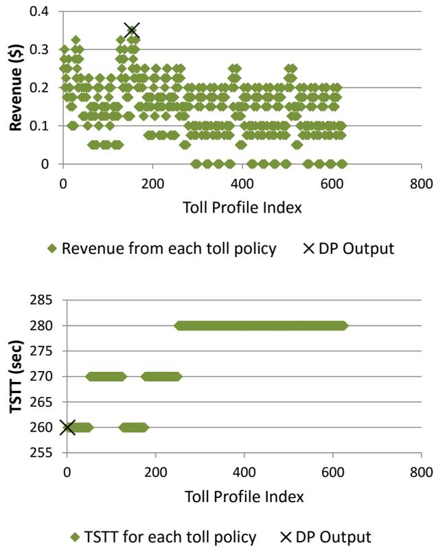
Figure 5.2: Plot of the revenue and the TSTT obtained from the DP algorithm compared against all the enumerated toll profiles
