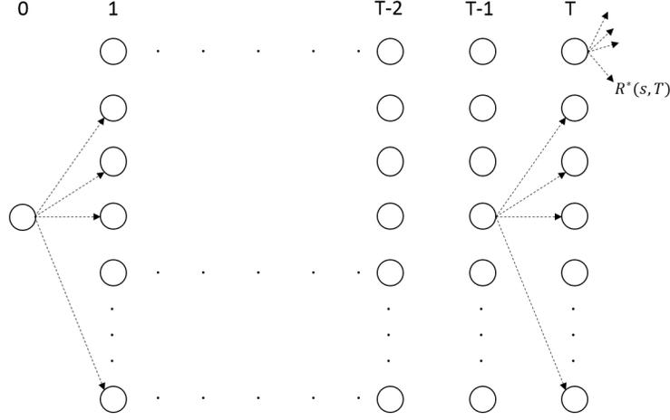
Figure 4.4: Pictorial representation of the backward recursion algorithm
