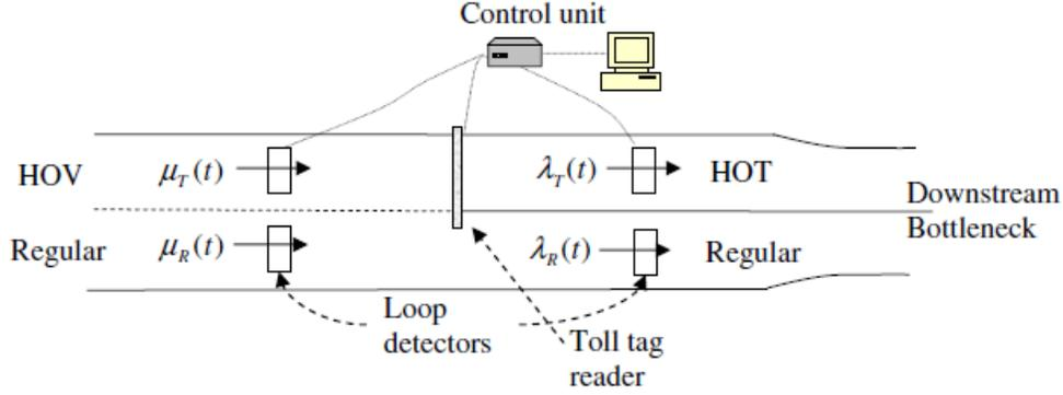
Figure 3.1: Loop detector locations (Source- Lou et al. [3])
