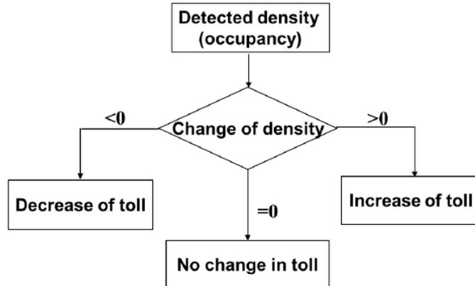
*Figure 1.2: Commonly used heuristics for dynamic tolling of managed lanes (Source- Michalaka et al. [2])*
