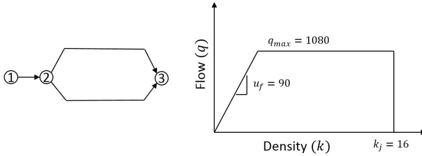
Figure 5.1: Single entrance single exit network used in simulation and the associated fundamental diagram
