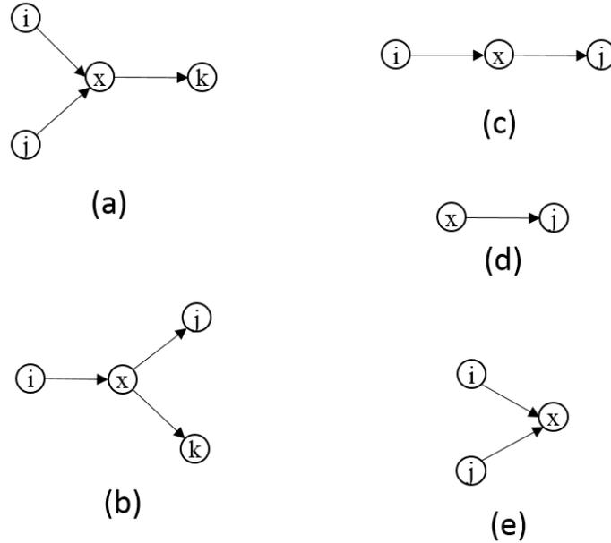
Figure 4.3: Possible types of nodes in a HOT system: (a) merge node, (b) diverge node, (c) series node, (d) origin node, and (e) destination node
