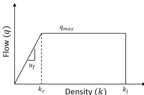
Figure 4.2: Spatial queue model fundamental diagram
