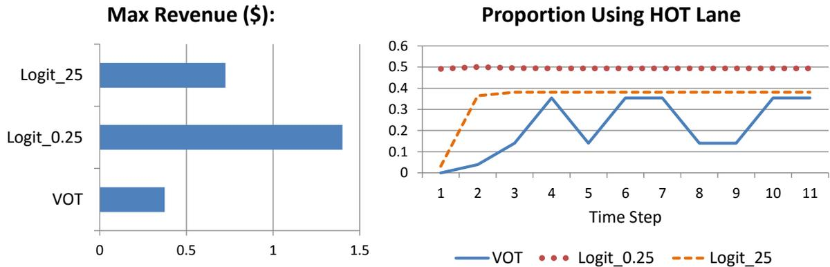
Figure 5.6: (a) Revenue collected from different choice models; (b) Proportion using the HOT lane predicted by each choice model at the optimal tolling
