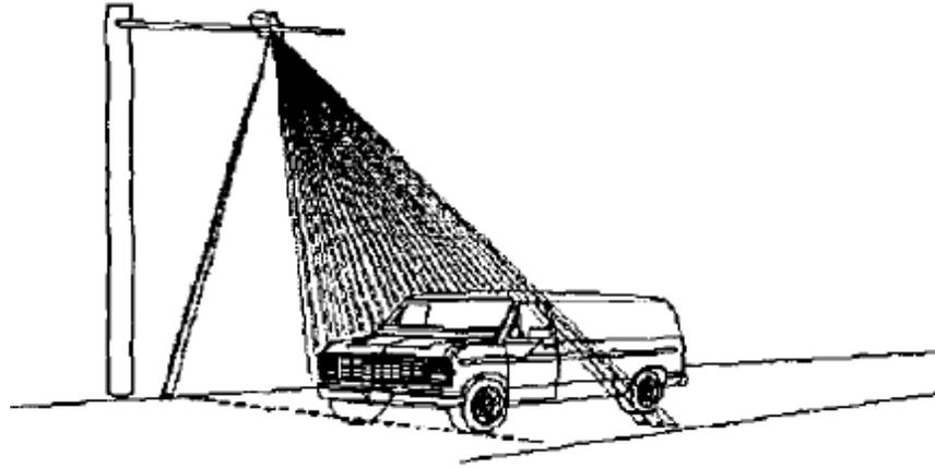
*Figure A.3: Laser detection technology*
