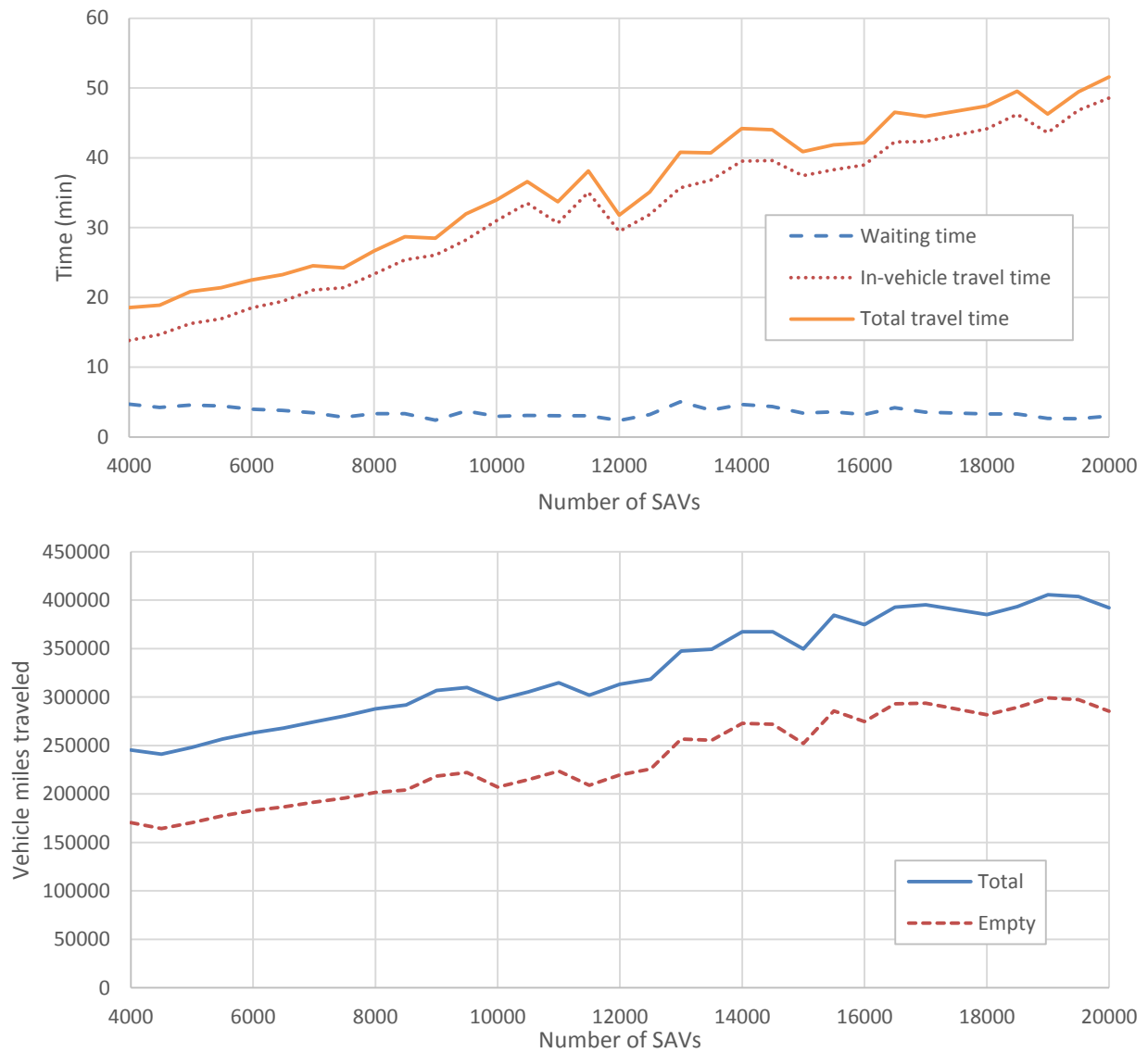
Figure 6: Travel time and VMT for the dynamic ride-sharing and preemptive relocation scenario
