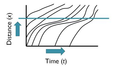
The density k is the rate trajectories cross a vertical line.
