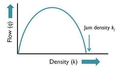
Also notice that there is some point at which flow is maximal. This maximum flow is the capacity  $q_{max}$ , which occurs at the critical density  $k_c$ .
