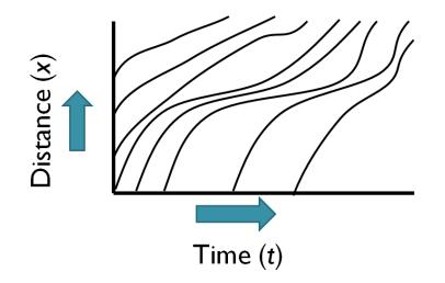
The flow q is the rate trajectories cross a horizontal line.
