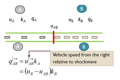
These flow rates should be identical, since vehicles are not appearing or disappearing at the shockwave. Thus
