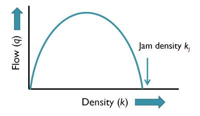
This is the *fundamental diagram*, denoted Q(k). The fundamental diagram can be calibrated to data, resulting in different traffic flow models.
