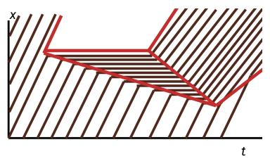
We can also define cumulative counts N as a function of x and t. While actual vehicle trajectories are discrete, we can "smooth" them so N(x, t) is continuous.
