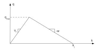
The main feature is a simplified fundamental diagram with only two wave speeds:  $u_f$  for the uncongested portion, and -w for the congested portion.
