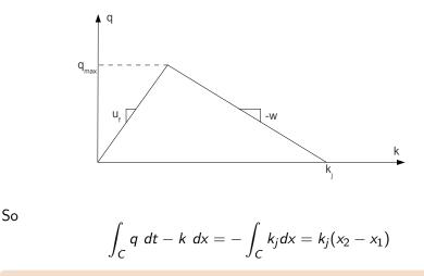
If you are moving at the backward wave speed, the cumulative vehicle count increases at the rate of the jam density.
