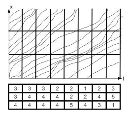
A roadway link is divided into "cells," and we track the number of vehicles in each cell at discrete points in time.
