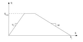
This diagram is defined by four properties: the free-flow speed  $u_f$ , the capacity  $q_{max}$ , the jam density  $k_j$ , and the backward wave speed -w.
