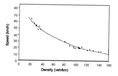
Collected in the (one-lane!) Lincoln Tunnel in 1959, based on a logarithmic fit to data  $(u \propto \log(k/k_i))$
