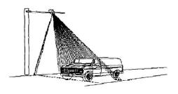
**Records:** Volume; speed (with two detectors), vehicle classification, lane position
