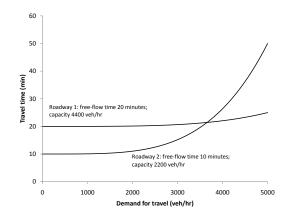
Each link performance function  $t_{ij}(x_{ij})$  is an increasing, convex function of the flow  $x_{ij}$  on that link alone.
