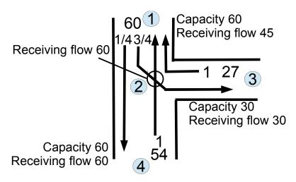
Sending flows and turning proportions shown. Links (2,4) and (2,3) have receiving flow of 60; link (2,1) has receiving flow of 45.  $\beta_{421}/\beta_{123} = 5$ .
