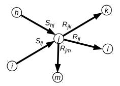
Like a diverge, the most restricted turning movement from each approach determines the flow to all of its movements. Like a merge, approaches competing for restricted receiving flow divide according to fixed proportions.
