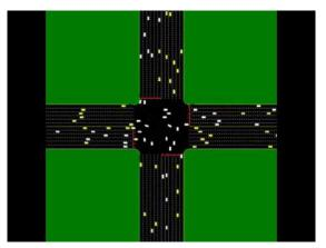
Microscopic models track the trajectories of individual vehicles at a very fine time scale ( $\approx 0.1$  seconds). They track the precise locations of each vehicles, account for variations in driver behavior, vehicle characteristics, and so on. This level of detail makes them highly realistic, but impractical for modeling large regions.
