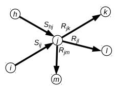
Like a diverge, the most restricted turning movement from each approach determines the flow to all of its movements. Like a merge, approaches competing for restricted receiving flow divide according to fixed proportions.
